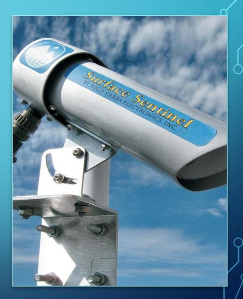
COMPONENTS FOR TEMPERATURE DETECTOR TYPICALLY LOCATED ON ROADSIDE OR THE JERSEY BARRIER
