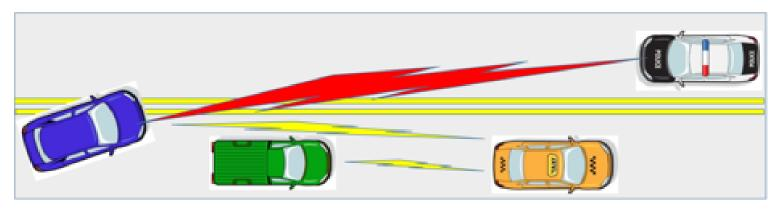
OBU from taxi transmits BSM that cab is moving slowly. OBU from blue vehicle transmits BSM that it is changing heading, potentially encroaching into pathway of police vehicle. Application Interface in police vehicle warns that blue vehicle may be encroaching into lane, while application interface in blue vehicle warns that there is an approaching vehicle (police car)
